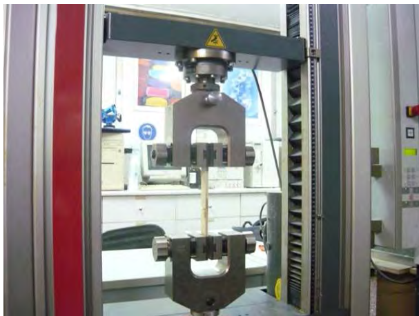
Testing of plywood for shear strength at Chimar premises
