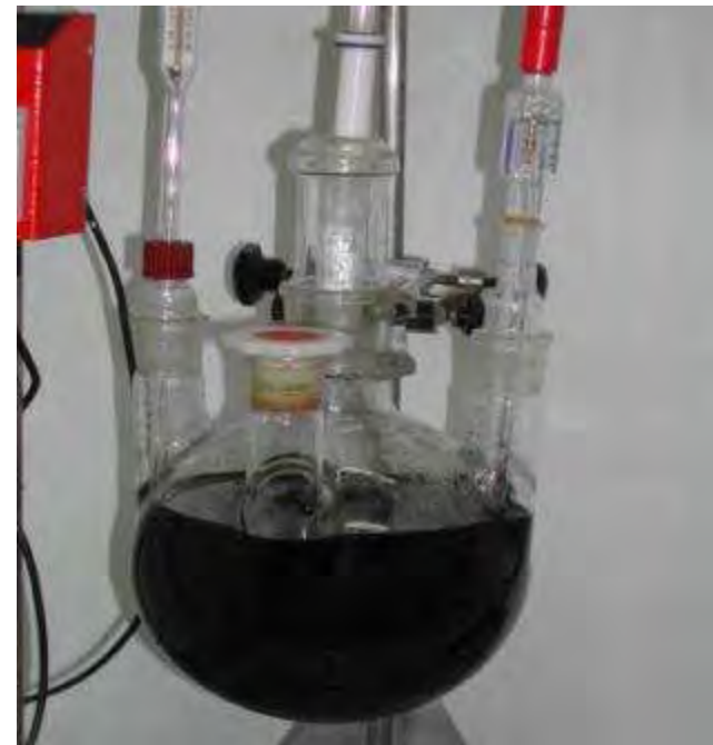
Lab synthesis of a PF resin at Chimar premises
