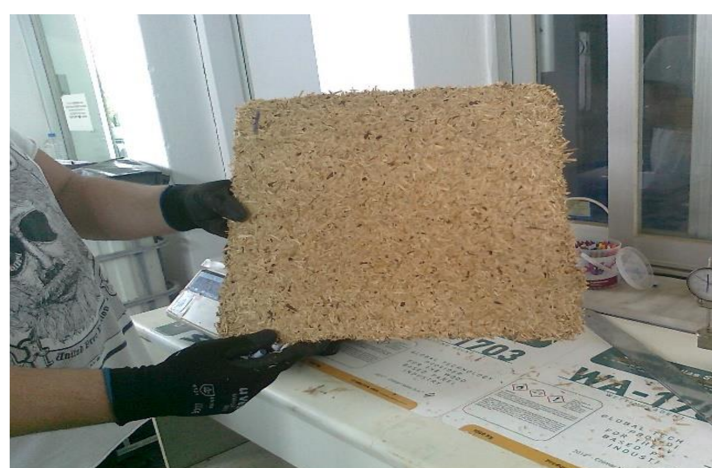
Figure 2. Particleboard made from milled wood pellets.
