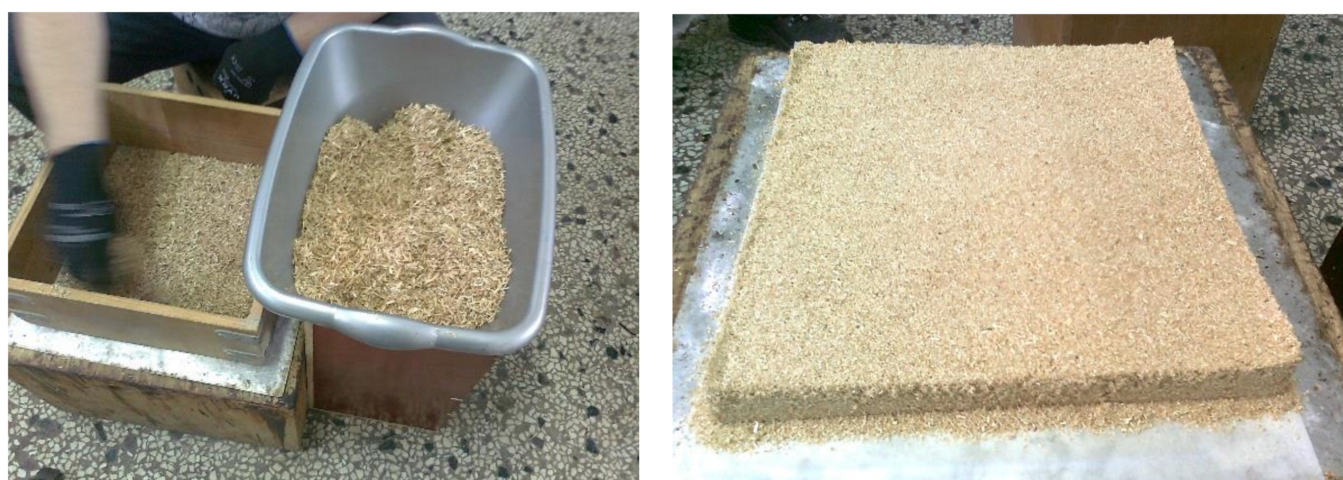
Figure 1. Making particleboard from milled wood chips.
