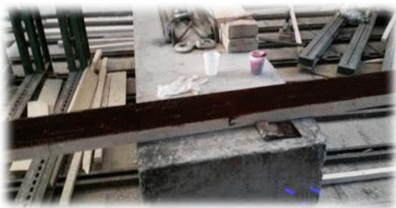
Picture 6: Spread PFL glue mixture on beam
