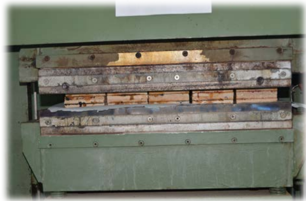
Picture 2: Laminated timber cold pressing
