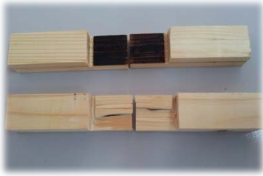
Picture 4: Laminated timber specimens after testing showing 0% and 100% wood failure
