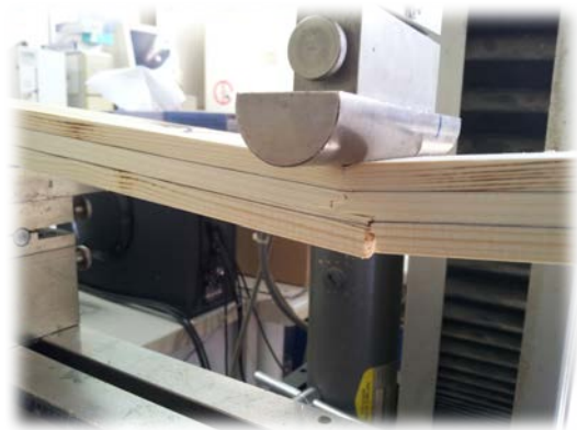
Picture 3: Testing of 3-lumber specimens (50 cm x 4cm x 2.7cm), 100% wood failure
