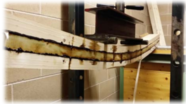
Picture 5: PFL-bonded glulam testing at TECNIFUSTA, Spain
