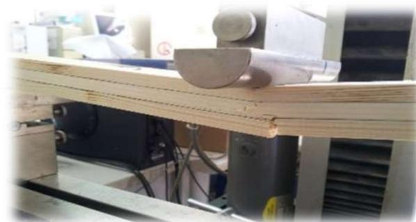
*Picture 2: Testing of 3-lumber specimens, 100% wood failure*
