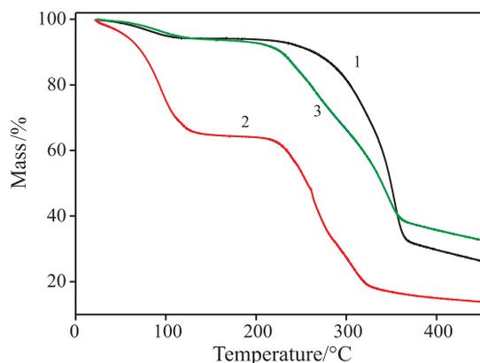
**Fig. 7** Mass (%) vs. temperature for 1 – wood chips, 2 – cured innovative resin and 3 – wood chips blended with the cured conventional resin
