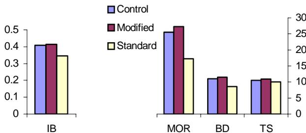
Figure 3: Tensile (IB) and bending (MOR) strength, 24h thickness swelling (TS) and bonding durability (BD) of pilot scale OSB produced with bio-oil modified PF resin.
