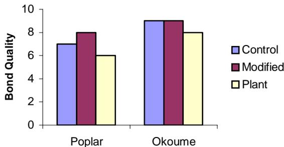
Figure 2: Bond quality of industrial plywood produced with bio-oil modified PF resin.
