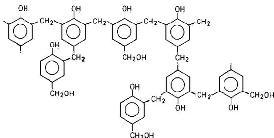
*Figure 1: Resole structure.*
